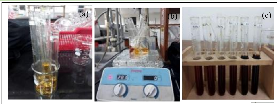
Fig. 2. (a) Before reaction, (b) Reaction process, (c) After reaction of DNS with glucose
