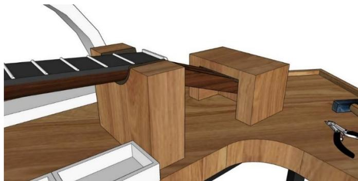
**Figure 10.** Guitar Head Lock and Guitar Neck Support
