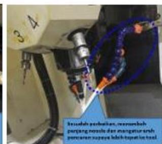
Figure 11. Nozzle coolant before and after
