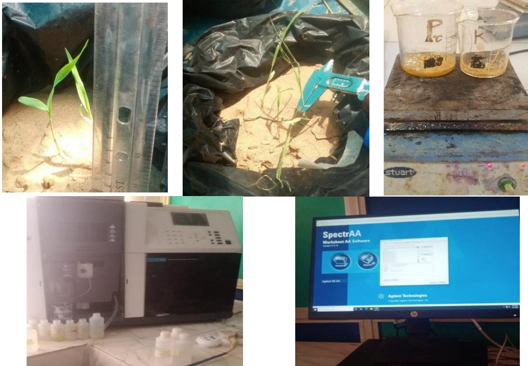
Fig. 2. Research Design (continued). Top left = measuring the growth parameters of the plants during the phytoremediation, centre = measuring the stem girth of the plants; c = digesting the soil samples for AAS; bottom left = AAS machine, right = SpectraAA software for AAS analyses
