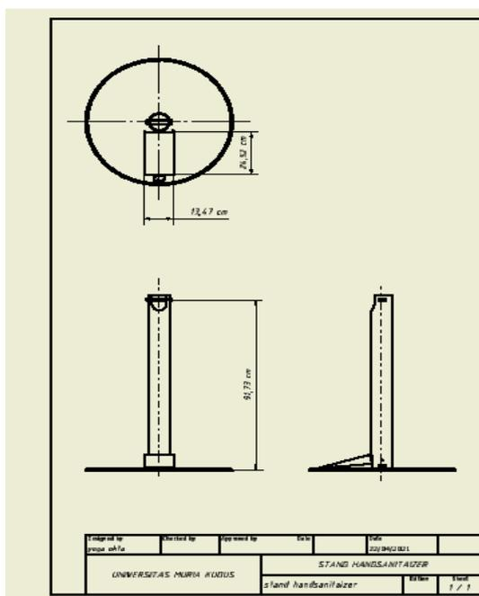
**Figure 4.** Engineering drawings of 2D ergonomic design of hand sanitizer dispenser stand
