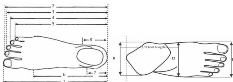
Figure 1. Foot dimensions measured (Hajaghazadeh et al., 2018)
