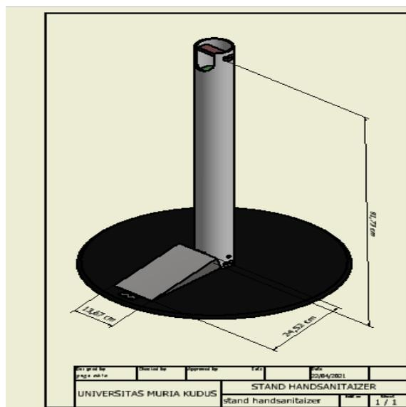
**Figure 3.** Engineering drawings of 3D ergonomic design of hand sanitizer dispenser stand
