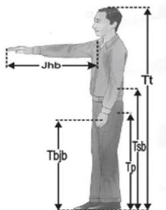
**Figure 2.** Body dimensions measured for standing position (Hari Purnomo, 2013)
