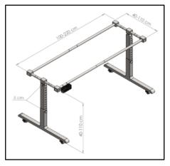
Fig. 9. Redesign of the Colet dyeing Table
