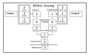
Fig. 11. REBA assessment for new design Colet table
