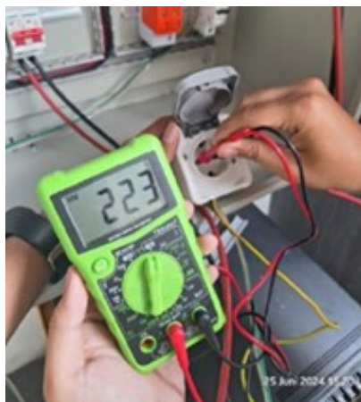
Fig. 8. Inverter voltage output
